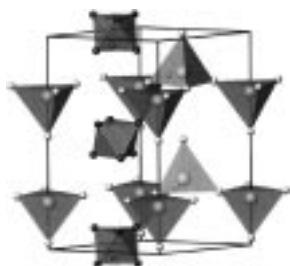
Figure 2. The structure of Ba 5 Ga 6 H 2 , with trigonal antiprismatic Ga 6 8- and hydride in barium tetrahedra.
