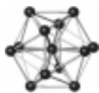
Figure 6. The \text{Tl}_{13}^{10-} cluster in \text{Na}_4\text{K}_6\text{Tl}_{13} .
