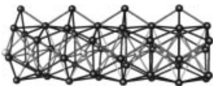
Figure 17. A portion of the infinite augmented chains of condensed cadmium-centered \text{Tl}_{10} antiprisms in \text{Cs}_5\text{Tl}_{11}\text{Cd}_2 .
